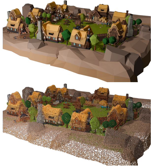
Figure 19. Applications on textured geometries. The setup is the same with Fig. 9. Top : ground-truth. Bottom : ours.
